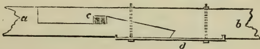
Fig. 95—Represents a scarf joint arranged to resist a cross strain and one of extension. The bottom of the joint is secured by an iron plate confined by bolts. The folding wedge key inserted at c serves to bring all the surfaces of the joints to their bearings.
